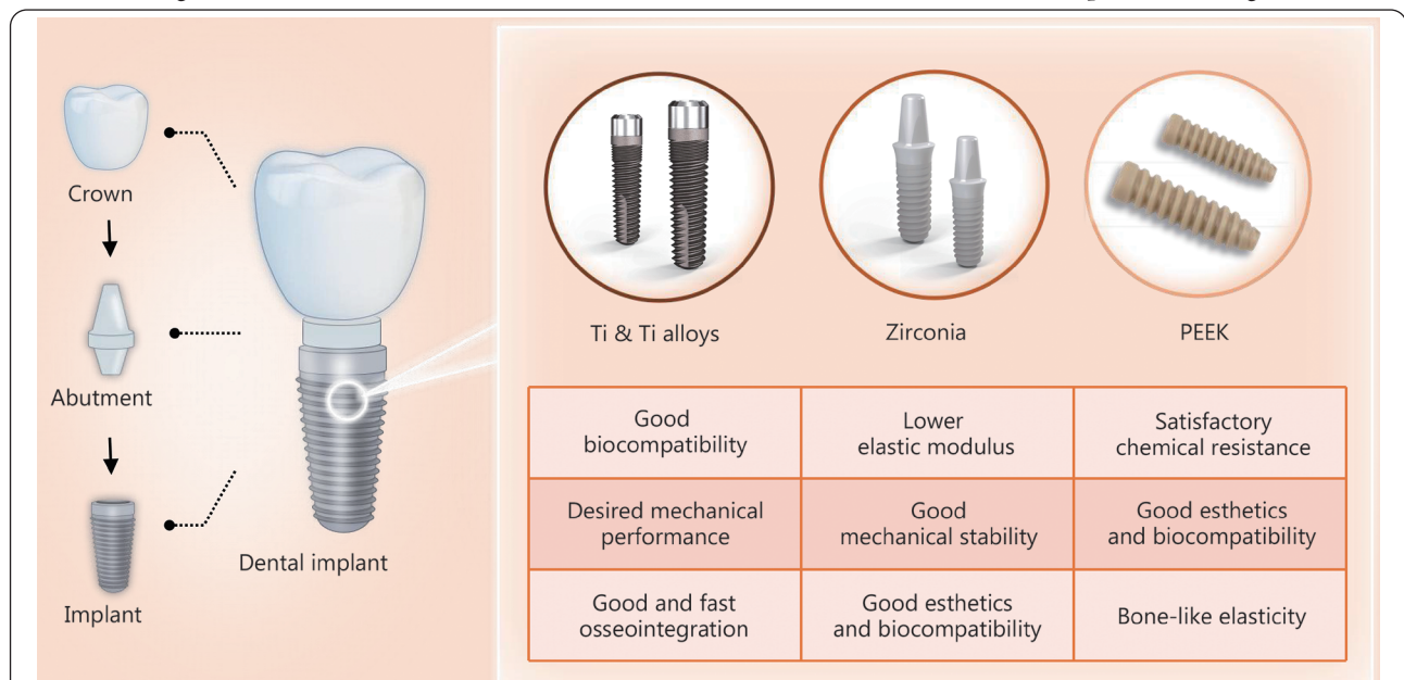
Fig. 1 Schematic illustration of structure composition of dental implant and the classification of dental implant biomaterials with their respective advantages.
