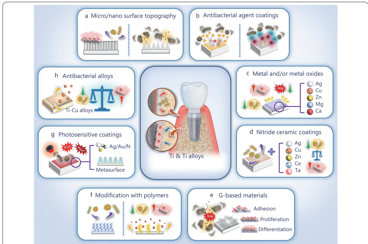
Fig. 5 Biomaterials and modification strategies for titanium (Ti)-based dental implants to enhance the osteogenic activities and antibacterial properties.
